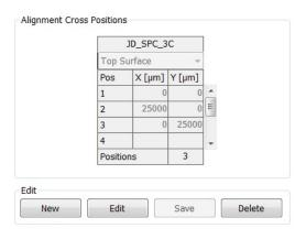
N. B. For back-side alignment exposure, make sure to remove the cache along the x- and y-axes of the table so that the back-side objective can detect the crosses at the back of the wafer.
