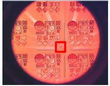
Press continue. Then, the edge detection script will find the edges of the wafer/chip, before continuing to the alignment/exposure steps.
