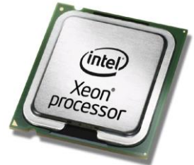
Intel Xeon [2006-] (820M trans., 3.73GHz, 64-bit, mem.:4MB/L2)
