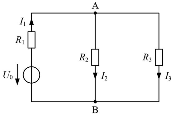
$$\begin{aligned}U_0 &= 4 \text{ V} \\R_1 &= 100 \Omega \\R_2 &= 100 \Omega \\R_3 &= 270 \Omega\end{aligned}$$
