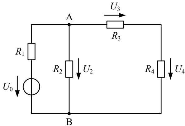
$$\begin{aligned}U_0 &= 4 \text{ V} \\R_1 &= 15 \Omega \\R_2 &= 270 \Omega \\R_3 &= 100 \Omega \\R_4 &= 100 \Omega\end{aligned}$$
