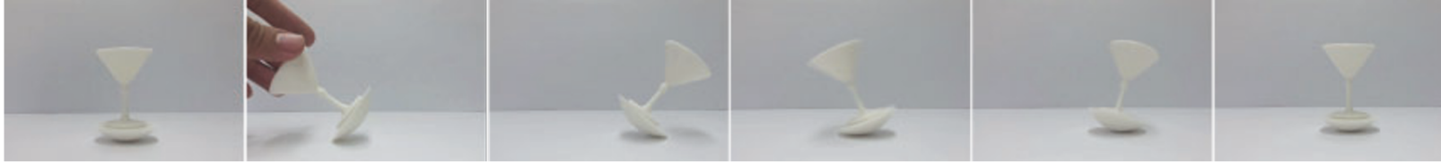
Figure 1: A goblet shape roly-poly toy example designed by our method. The snapshots show that the toy is able to regain balance when pushed over.
