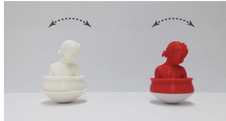
Figure 1: A goblet shape roly-poly toy example designed by our method. The snapshots show that the toy is able to regain balance when pushed over.
