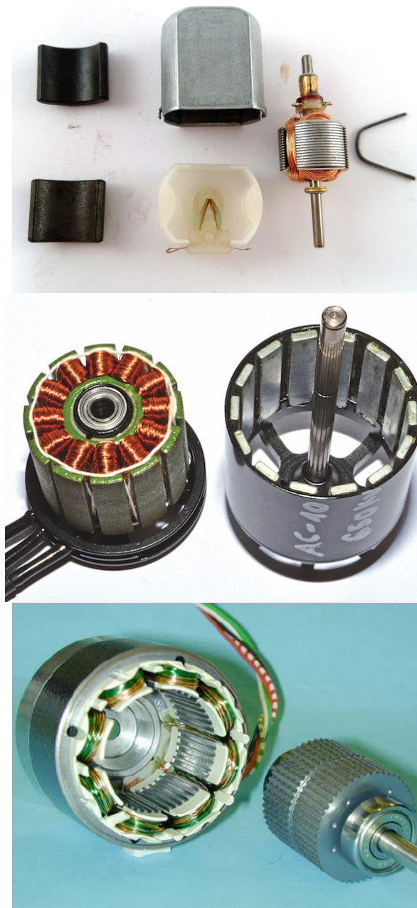
Figure 35.1: A brushed motor (top), a brushless motor with an external rotor (center), and a bipolar stepper motor (bottom), all opened up.
