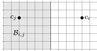
Figure 2.12. The shape of \mathcal{B}_{i,j} for AWGN channels and ML decision.
