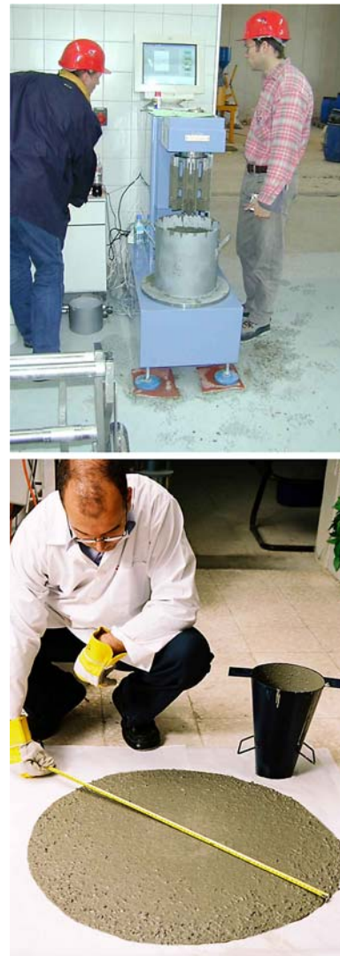
Fig. 3 Viscometer used for determining rheological material data and workability testing in practice (Courtesy of M. Sonebi)
