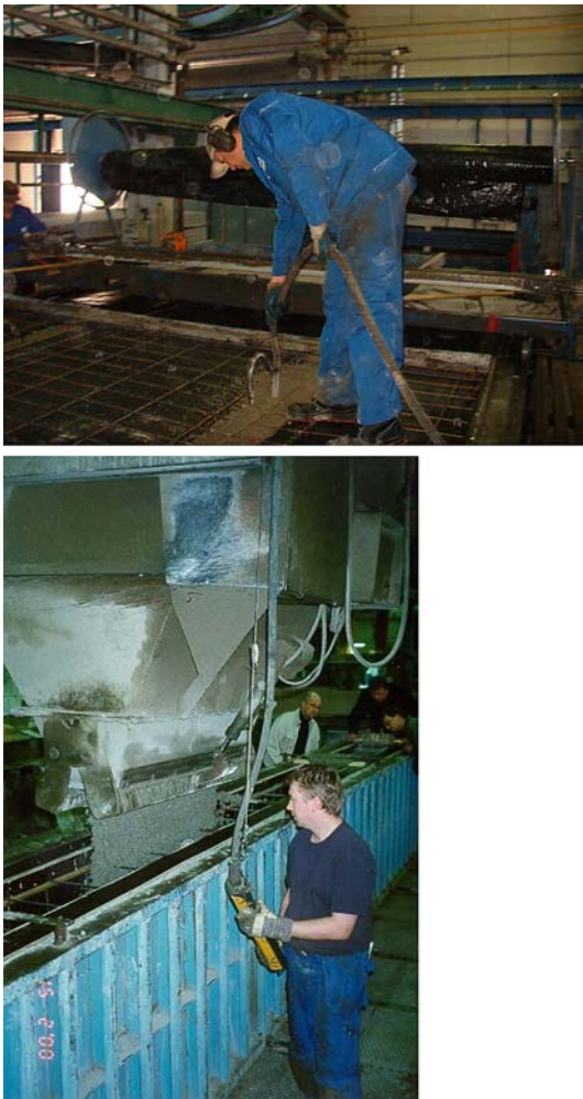
Fig. 14 From noise, vibration, ergonomic loading to high quality working environment using self-compacting concrete (SCC) in precasting (Courtesy of K. Juvas)
