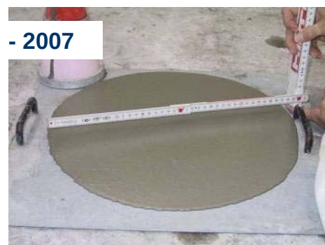
UHPFRC with CEM I 52.5 (Salonit), 50 % replacement by Limestone Filler
