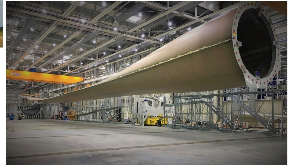
107 meters, LM Wind Energy's blades for the Haliade-X, 12MW
