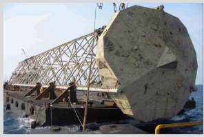
Jack-up drilling leg (after ConocoPhillips)
