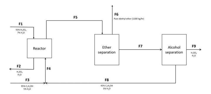
If there is an 87% single-pass conversion of the ethyl alcohol fed to the reactor, calculate:
