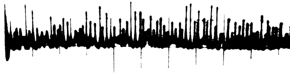
FIG. 8.2. Typical time behavior of early cw-pumped solid-state lasers. Time scale is 50 \mu\text{s}/\text{div} . (after reference, (3) by permission).
