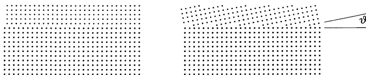
Figure 5.21: Untilted (left) and tilted (right) epitaxy.
