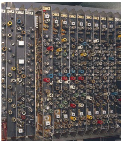
An early stored-program computer (left), built around 1950, used vacuum tubes in logic circuits, whereas modern computers use transistors and silicon wafers (right), but both are based on the same principles.
